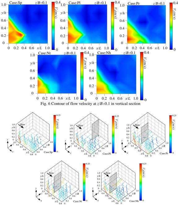
Fig. 7 Vector of flow velocity at nearly partition
