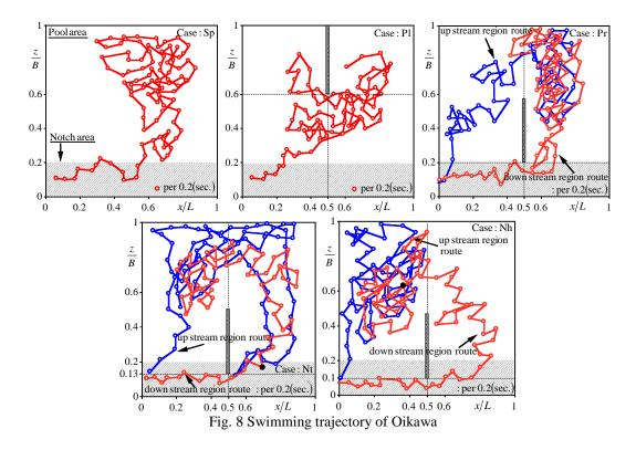
other cases. In Case (Nt) and (Nh) that were installed partition between upstream side notch and down one. Therefore, water fall conflicts with partition and it is reduced.
